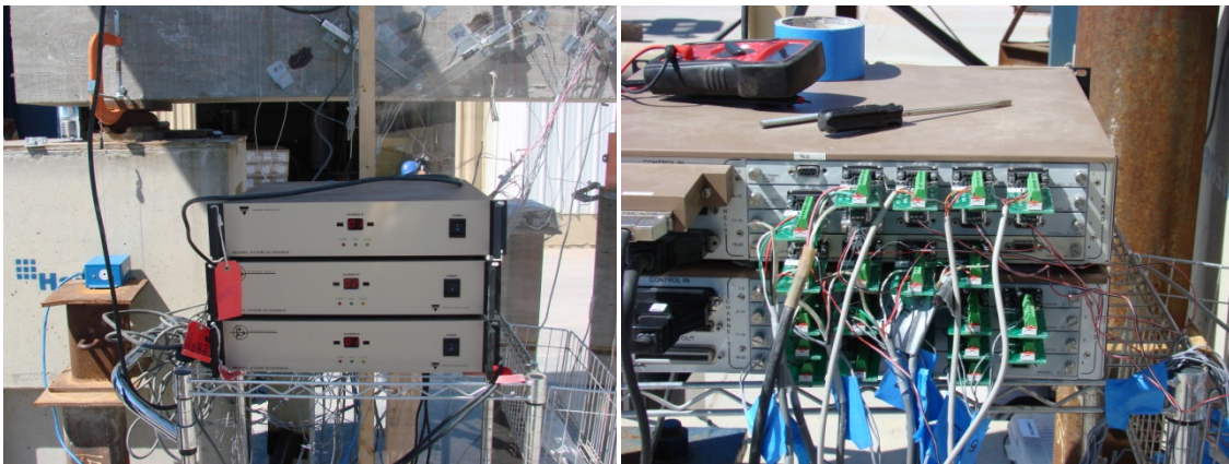
Figure 3.16 Vishay 5000 DAQ system
