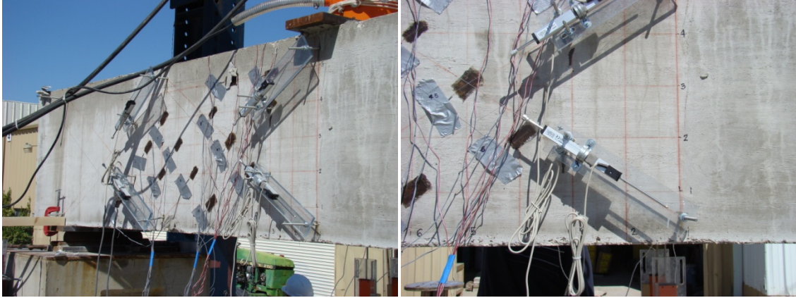
Figure 3.22 Typical instrumentation of diagonally placed LVDTs
