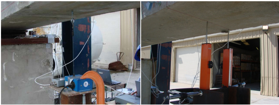
Figure 3.23 LVDTs for measuring deflection: (a) String pot; (b) Rod type of LVDTs
