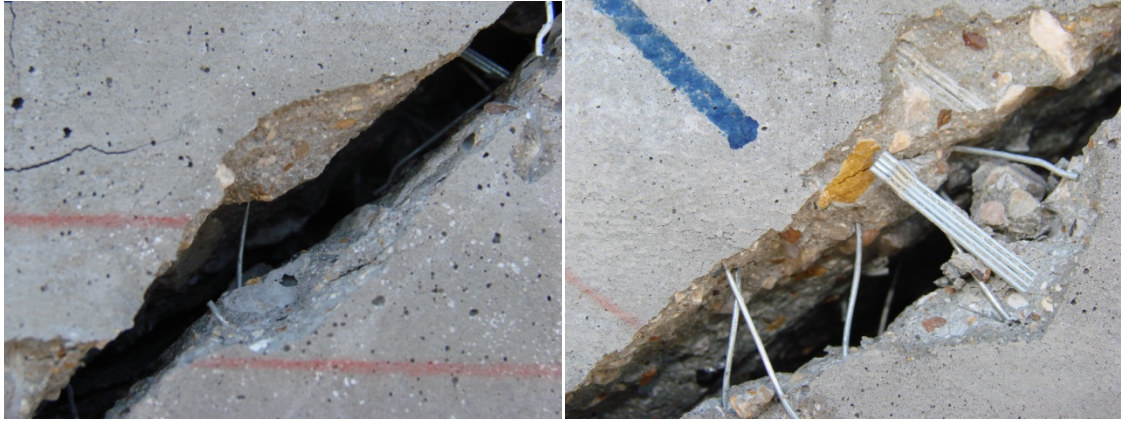
Figure 3.25 Poor fiber distributions due to undissolved glue
