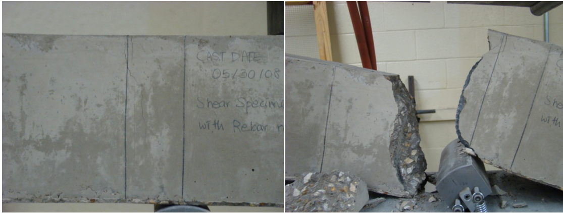
Figure 4.27 Test results of the specimen with C- shaped rebar reinforcement; (a) Initial crack; (b) At failure
