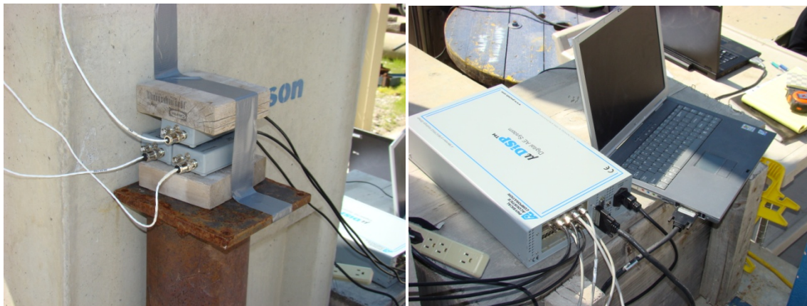
Figure 6.12 AE DAQ system; (a) pre-amplifier; (b) AE DAQ system
