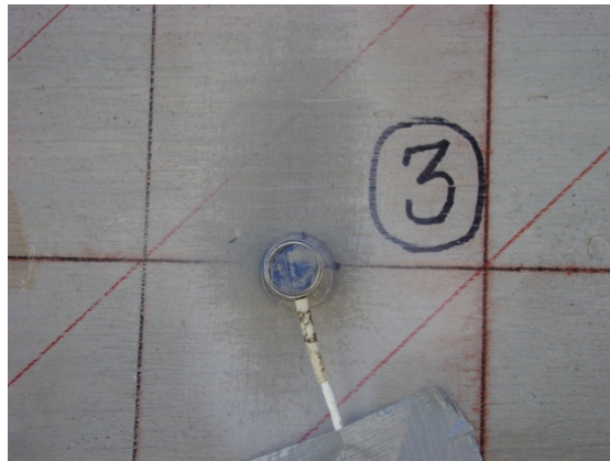
Figure 6.11 AE sensor instrumentation
