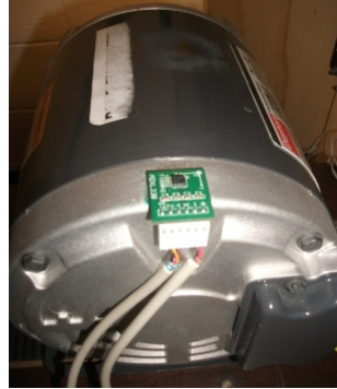
Figure 4.3 ADXL330 Tri-axial Accelerometer Mounted on the Motor Housing
