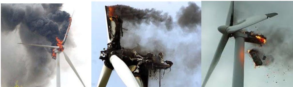
Figure 1.1 Catastrophic Failure of a Wind turbine due to Lack of Proper Monitoring System
