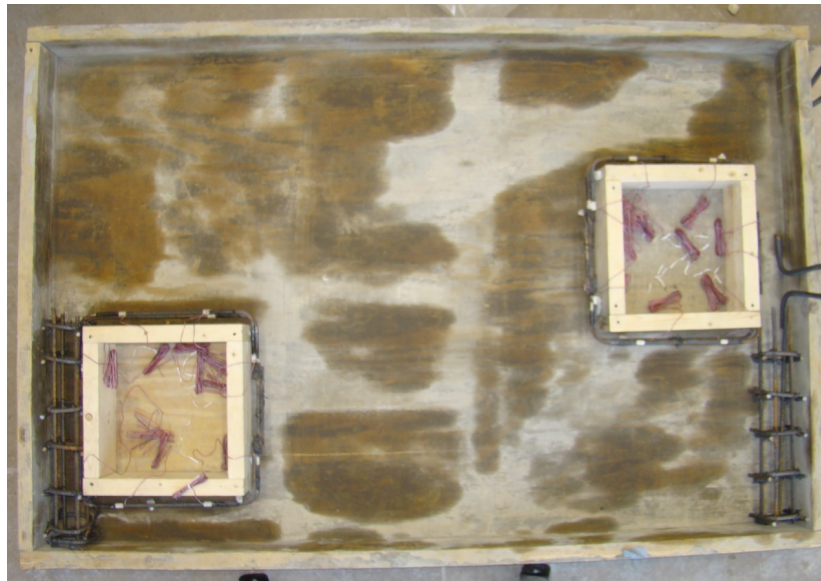
Figure 4.26 SFRC #1 specimen reinforcement layout (Numbers on the bar indicate strain gauge number and letter indicating type of layer "T"- top and "B"- bottom)
