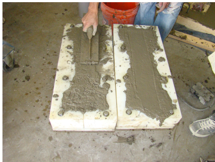
Figure 3.28 Final touch given to dog-bone specimen after installing four layers of mesh
