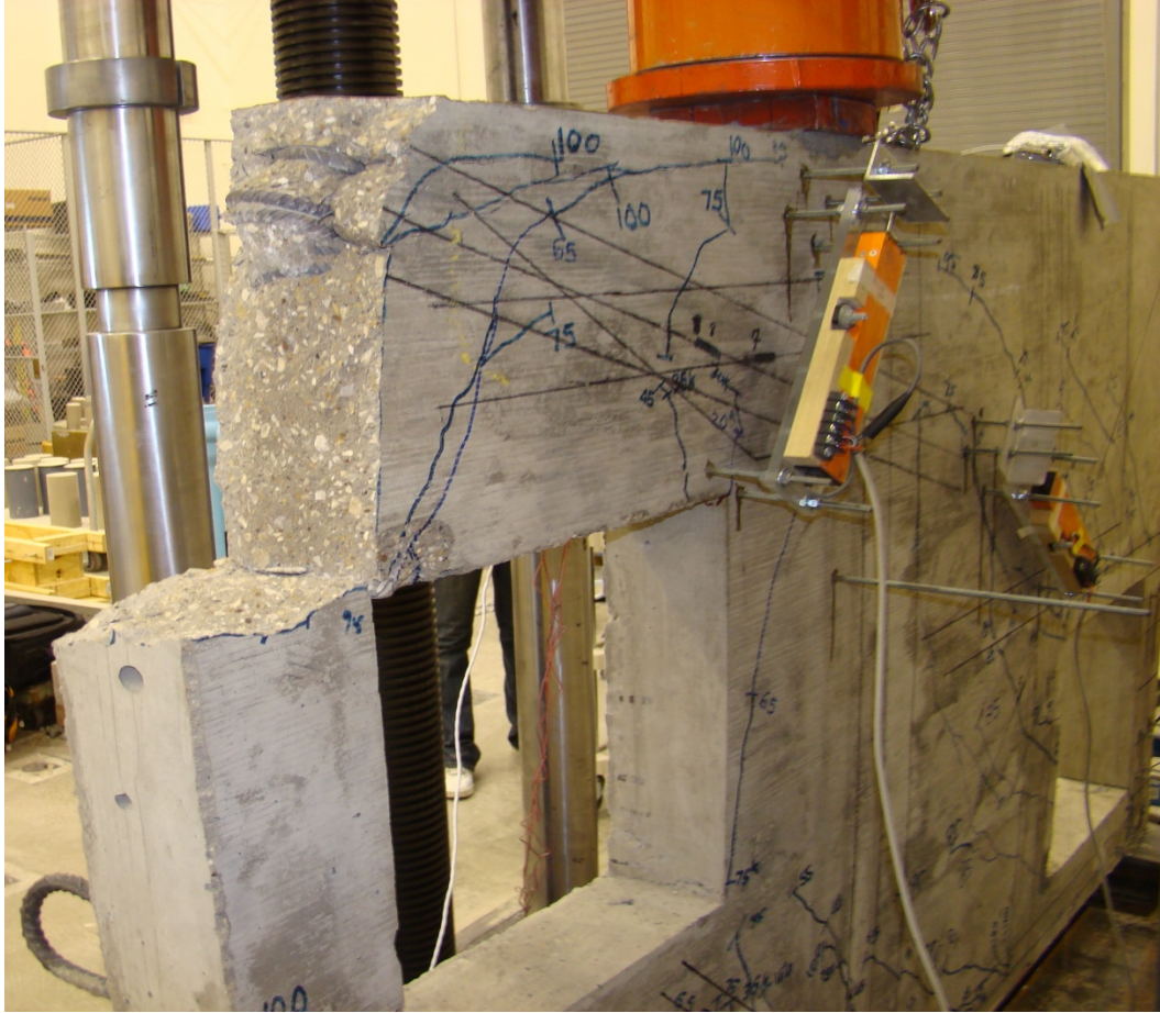
Figure 4.18 Top right corner of RC specimen at 100 kips
