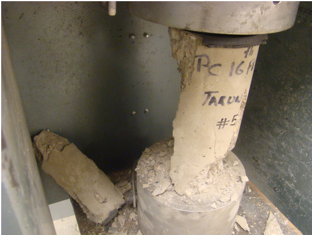
Figure 3.4 Typical plain concrete cylinder after testing
