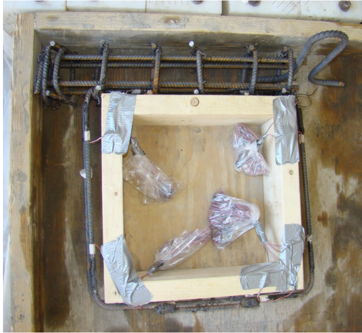
Figure 4.28 Square loops of reinforcement around the window, cage at support and anchor bar in SFRC #1 specimen
