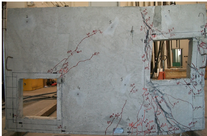
Figure 5.39 Overall state of SFRC#3 specimen after testing
