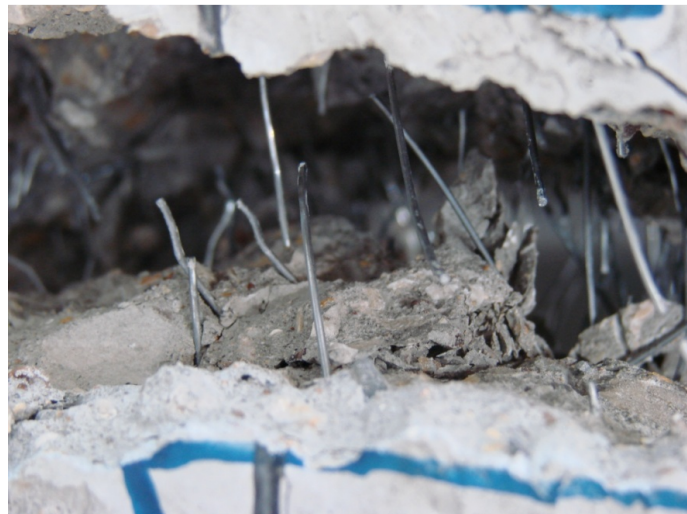
Figure 4.39 Fiber pull out at failure of SFRC #1 specimen
