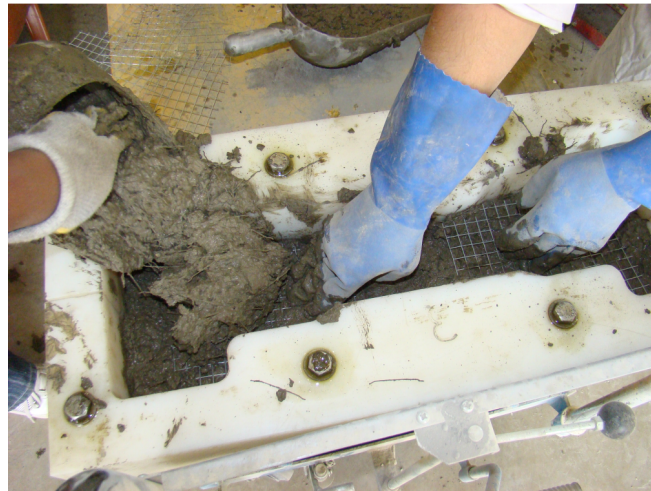
Figure 3.27 Placement of wire mesh in end section of dog-bone specimen
