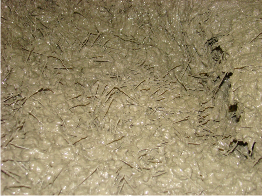
Figure 4.30 Close up of concrete mix with fiber for SFRC #1 specimen
