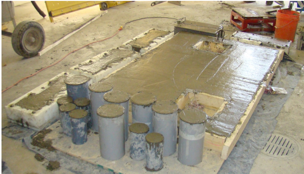
Figure 4.55 Finished SFRC#2 specimen and material specimens after casting
