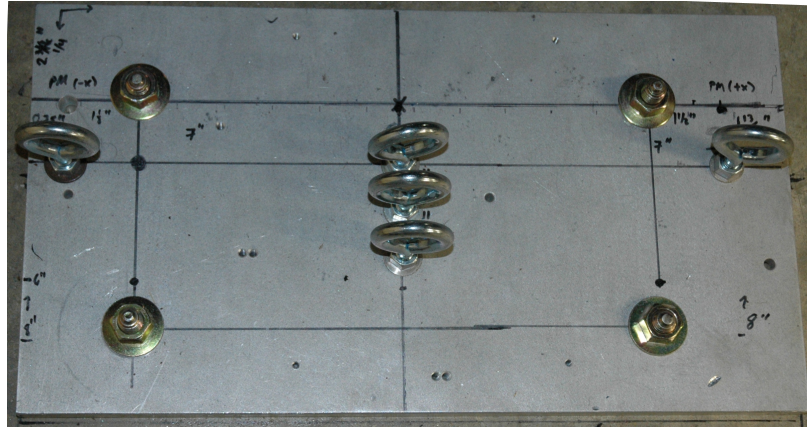
Figure 3.3. The plate that was manufactured for applying the static loads to the force balance.
