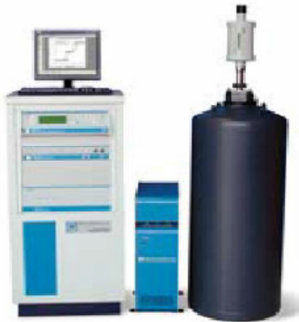
Figure 3.5 Quantum Design PPMS with VSM insert.
