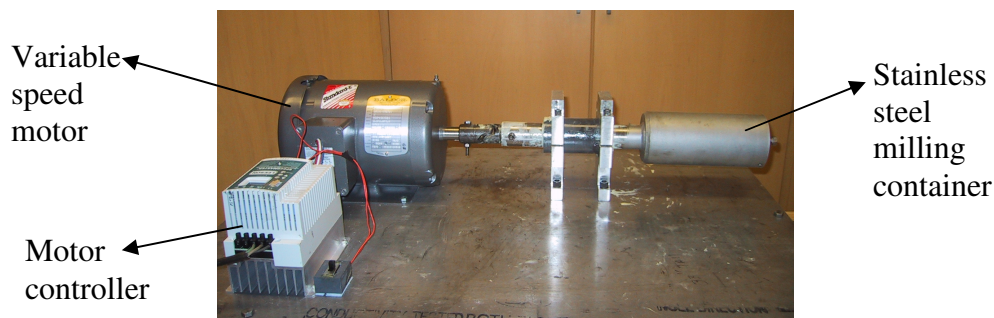
Figure 3.1 The ball milling set-up for milling of NaCl powder
